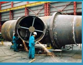
Fabrication Main Circulating Water Piping for Đăk Glun Hydropower Plant
