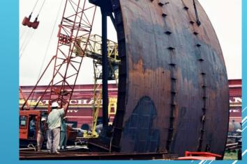
Fabrication Gate Valve for Đăk Gluk Hydropower Plant
